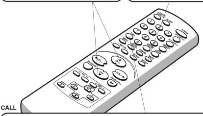
Press the CALL button. The clock, date, channel number, real time tape counter, tape speed and VCR operation will be indicated.
